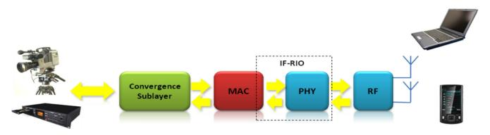
The command/control PHY/MAC interface of WisyMAX-RT is based on the Intel PHY-SAP for IEEE 802.16e as protocol while a standardized data structure allows for communication across PHY and MAC levels.
